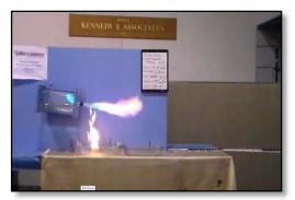
Fluid beginsejection as flame enters vessel. *c*)
