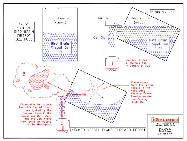
Figure 1. Illustration of the principle of the "Necked Vessel Flame Thrower Effect" from an actual litigation involving refill decorative fire pot gel fuel.
