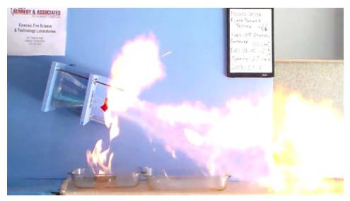
*Figure 4. In Test 66, a steel restrictor plate was attached to the opening of the flask. The ejection velocity increased dramatically compared to the normal (larger) opening.*
