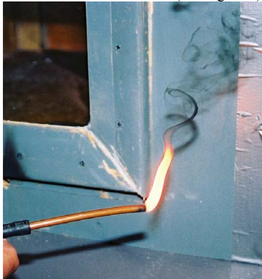
Figure 4 – Smoke Source, 2” laminar MAPP Gas flame
