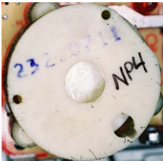
Figure 9 – Lack of Acoustic Soot Agglomeration on the horn enclosure of a non-powered smoke alarm
