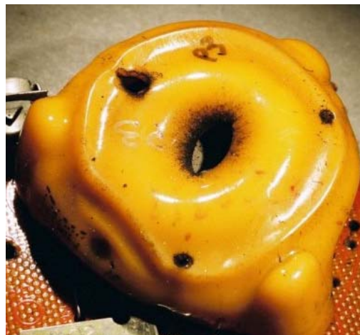
Figures 13 a. and b. – Patterns Persistence Soot agglomeration on a horn enclosure central sound exit opening before (left) and After (right) heating to 433° F. (223° C) for thirty minutes
