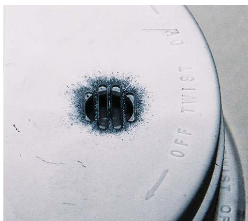
Figures 10 a. and b. – Acoustic Soot Agglomeration around the sound exit grillwork of a Kidde Smoke Alarm
