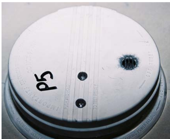
Figures 10 a. and b. – Acoustic Soot Agglomeration around the sound exit grillwork of a Kidde Smoke Alarm
