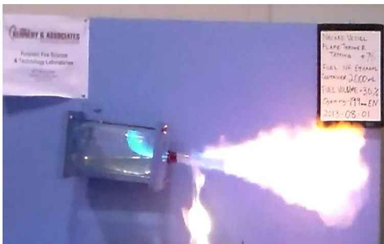
Figure 1. Necked Vessel Flame Thrower Effect test at JAK&A Laboratories.
