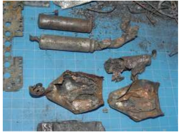
Figure 11. Remains of laptop battery from in a fire scene. Each Li-ion cell displays a different degree of damage.
