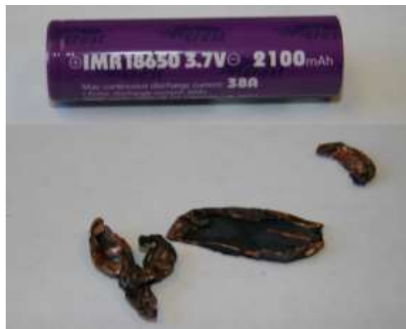
Figure 1. Lithium-ion 18650 cell, and a failed cell that exploded in a victim's pocket.
