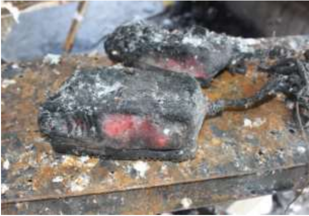
Figure 10. Charger/battery remains in the area of origin. Found to be Ni-Cad battery, not Li-ion.
